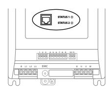
The RJ45 port has some terminals that are internally connected in parallel with the pluggable control terminals as shown below:
