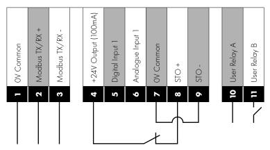
STO signal must be provided in order to permit running the motor. Start/Stop commands and speed reference are provided by serial communication. In Modbus mode, the digital input and analogue input can be used as remote I/O by the controller, the relay output can also be configured to be controlled by Modbus and used by the controller if required. In Modbus mode, the drive can be re-set from a fault by toggling bit 3 of the command word.
