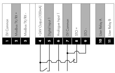
STO signal must be provided in order to permit running the motor. Start/Stop command provided by the Digital Input (P1-11 = 1) or when the analogue input level is greater than 1% (if P1-11 =2) and speed reference provided by the Analogue input. The drive can be re-set from a fault by removing and re-applying the digital input.
