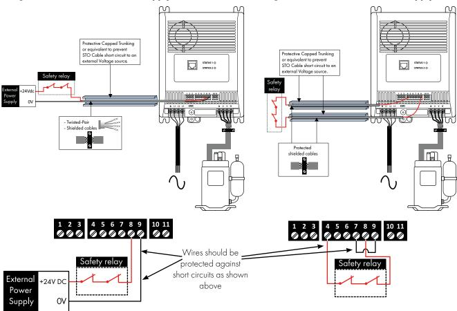
NOTE The Maximum cable length from Voltage source to the drive terminals should not exceed 25 metres.
